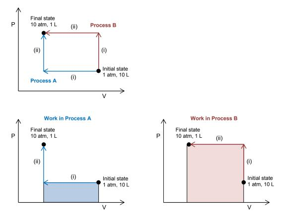
From the P-V diagram, it is clear that the more work is done by the system is in Process B.
