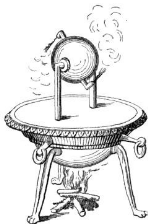
Aeolipile The first steam engine
